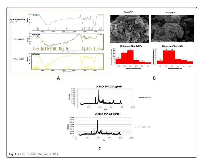
arene), alkane (OCH<sub>3</sub>), the methoxylic at  $1188.54 \text{ cm}^{-1}$ , and C-O stretching at 1025.79 appeared in the IR spectrum of complex as shown in Fig. 2a.
